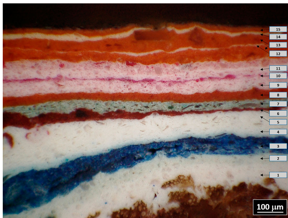
Figure 3. Digital micrograph of a cross section sample from The Big Egg . The sample was used in SEM-EDS elemental maps. The numbers of the layers from ground (1) to top layer (15) correspond to the numbers of layers presented in Table 1.
